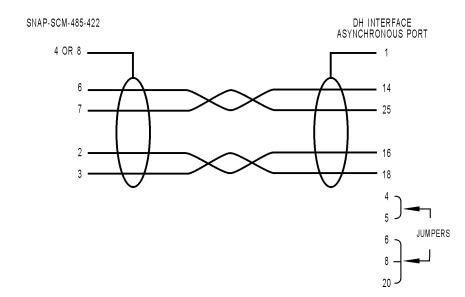
Opto 22 RS-422 serial connection to DH interface device:
