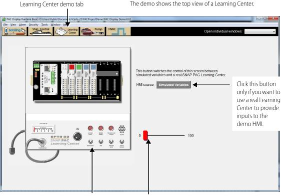
Turn LEDs on and off by clicking these toggle switches.
