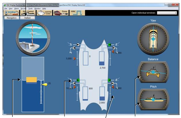
Total ship weight is shown by orange plus blue boxes. Blue represents total ballast. Vertical placement shows draft as a result of total ship weight. Push the On/Off buttons to fill and drain ballast tanks.
