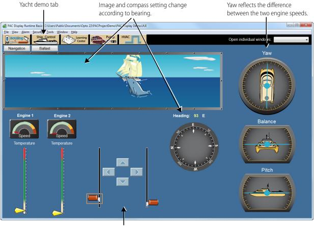
Move the speed controls to change yaw and bearing.
