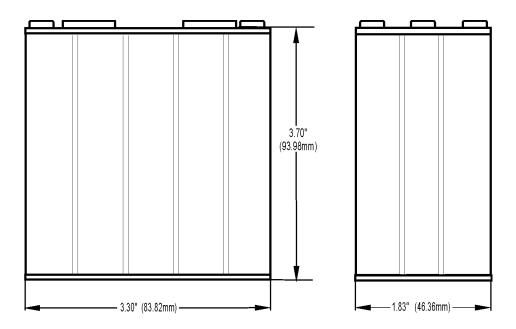
NOTE: The Arbiter and the Redundant Power Switch can be mounted on a panel or a DIN rail. For DIN-rail mounting, purchase one DIN-rail mounting kit (part number SNAP-ROKDIN) for each device. The DIN-rail clip adds an additional 0.375 inches (0.95 cm) to the device's height.
