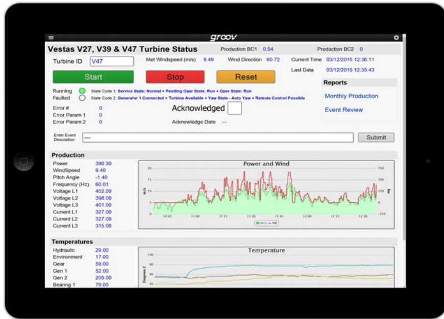
Opto 22’s groov interface makes it easy to monitor and control wind turbines from anywhere using a smartphone or other mobile device.
