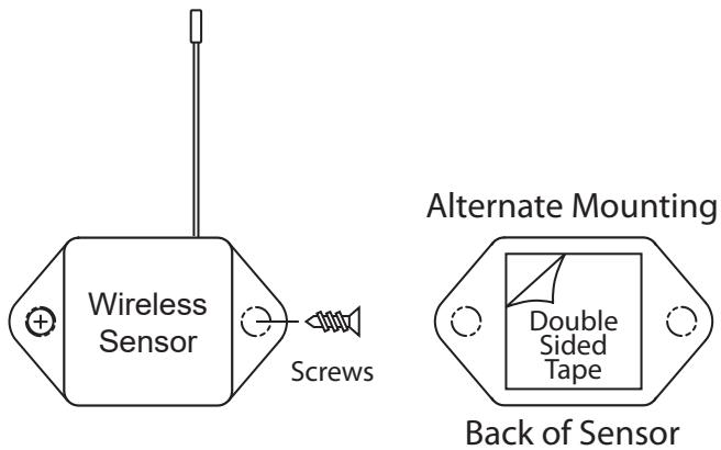
In order for your wireless sensors to work optimally, you should orient all antennas for your sensors and gateway(s) the same direction (typically vertical). Also sensors must be at least 3 ft. away from other sensors and the wireless gateway in order to function properly.
