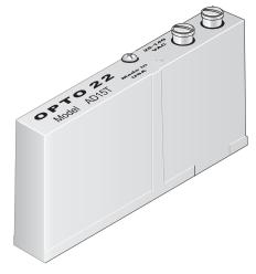
appropriate voltage transformer. The module reads the average voltage. Fusing the input lines is recommended. Modules plug into any Standard Analog I/O mounting rack and are secured by a captive screw. Field connections to the module are made via terminals located on top of the module.
