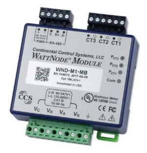
The WattNode® Meter Module measures bi-directional energy, power, voltage, current, etc. It communicates using Modbus® RTU over RS-485. The Meter Module provides revenue-grade system accuracy when used with the CCS Accu-CT® family of revenue grade (C0.6 or better) current transformers.
