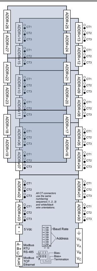
Figure 1: Connection Diagram
