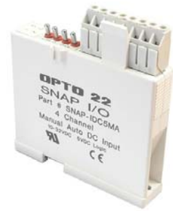
Input module with manual/auto switches
