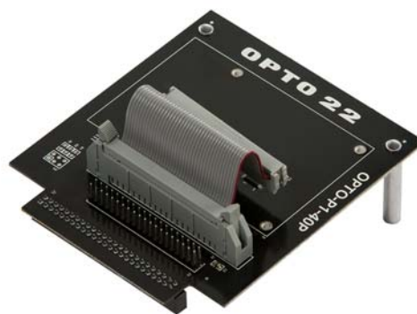
Digital I/O Carrier Board for Raspberry Pi
