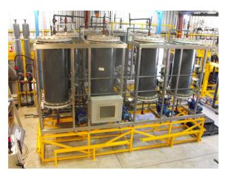
Biomass SMB for recovery of basic sugars from cellulose waste
