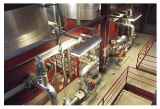
Simulated moving bed (SMB) for molasses (sugar recovery)
