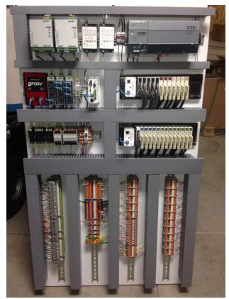
Opto 22 PACs and I/O provide control and monitoring capabilities for ARi systems. Opto 22's *groov* provides remote monitoring and control, a common customer request.
