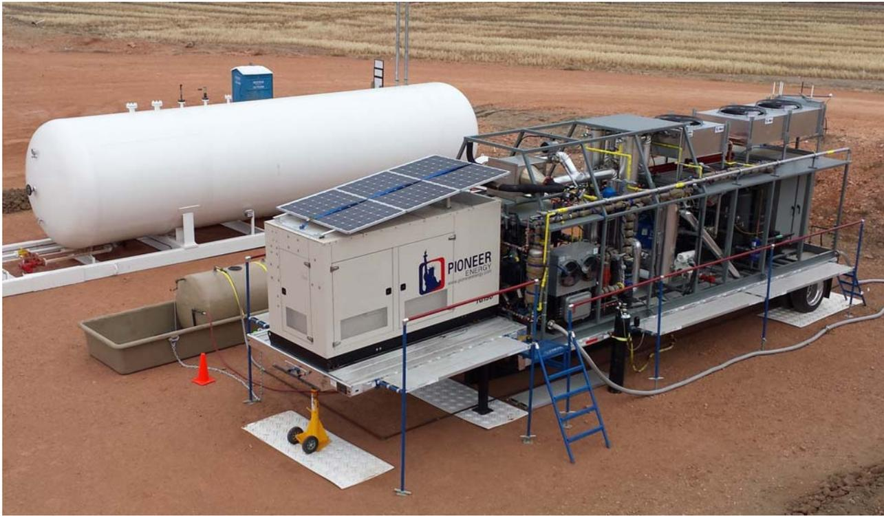
*Pioneer Energy's MAGS system is shown here deployed at a well site in North Dakota. Processed gas is stored in the large tank.*
