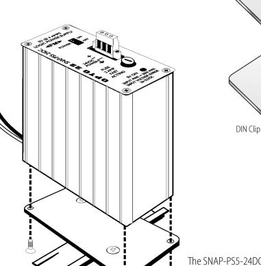
The SNAP-PS5-24DC power supply is shown in this example. Other devices have similar base plates.
