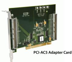
AC5 and PCIe-AC5 cards include four LEDs that can be used for debugging or indicating application status.
