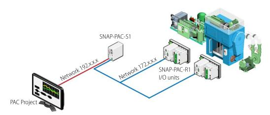
In this example one of the PAC's network interfaces is connected to the control network and the other to the computer network. If you're using PAC Project on the computer network, you can communicate with that PAC. But you cannot communicate directly with a different PAC that is wired only to the control network.
