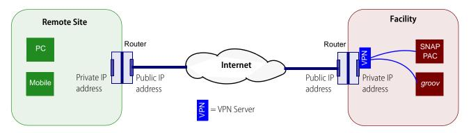
In the router, set up a port forward rule so the router will know to send data through the proper port to reach the VPN server. Port numbers depend on the VPN protocol you're using:
