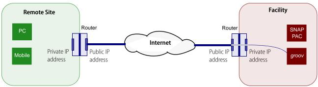
**Port forwarding** creates a hole in your firewall to allow certain packets through. PF works for *groov* because *groov* requires authentication from all users.
