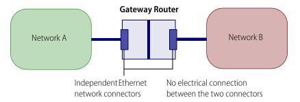
Software rules (routing tables, network address translation) determine whether and how communication moves between Network A and Network B.
