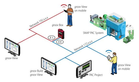
In this example, your *groov* Box is connected to your company computer network using Eth0 and to your control network using Eth1. (You could do the same thing with *groov* Server for Windows running on a PC that has two network interface cards.)
