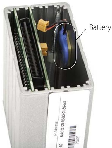
5. Notice the battery's position. Carefully pry the battery off the wall. (An R-series PAC is shown as an example.)
