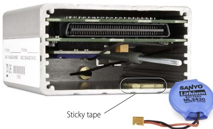
6. Carefully scrape the remaining sticky tape off the metal wall.
