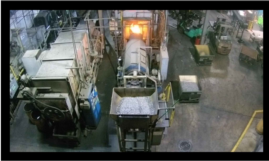
groov View HMI—camera feed of feeder hopper level
