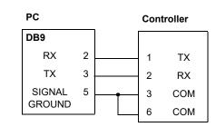
\* Minimum requirements for wiring an RS-232 serial cable to connect to a PC. If you want to connect the controller to a modem, see form #1595, the *SNAP PAC R-Series Controllers User's Guide*, for all eight pin connections.
