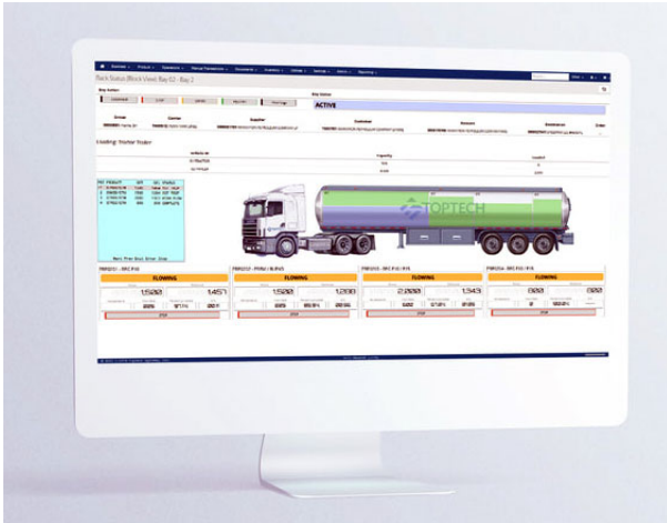
A terminal automation system (TAS) monitoring screen
