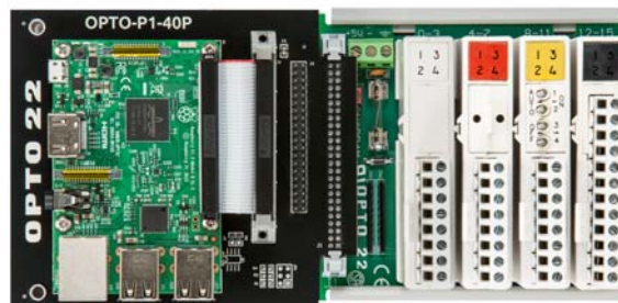
Digital I/O System for Raspberry Pi —This example shows a Pi, the Digital I/O Carrier Board, and a SNAP mounting rack with four 4-point SNAP digital I/O modules, totalling 16 I/O points. All items are sold separately.
