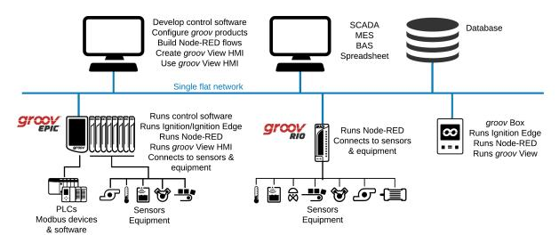
Adding mobile devices. For users on mobile devices, you can add wireless access points. With a WiFi connection, authorized users on tablets and phones can also configure *groov* EPIC and *groov* RIO and use your HMI. Authorized users on laptops with WiFi can do the same things as a user on a wired computer.
