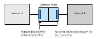
Software rules (routing tables, network address translation) determine whether and how communication moves between Network A and Network B. In addition to managing communication between LANs within your facility, a gateway router is also used to manage communication between a LAN and a WAN (wide area network). A WAN may be private or public; the internet is a public WAN.
