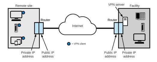
Most current PCs and mobile devices have VPN client software built in. The VPN client must use the same VPN protocol as the VPN server. Some clients give you a choice.
