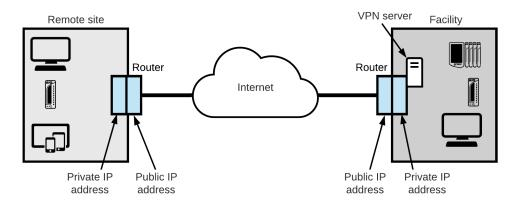
In the router, set up a port forward rule so the router will know to send data through the proper port to reach the VPN server. Port numbers depend on the VPN protocol you're using:
