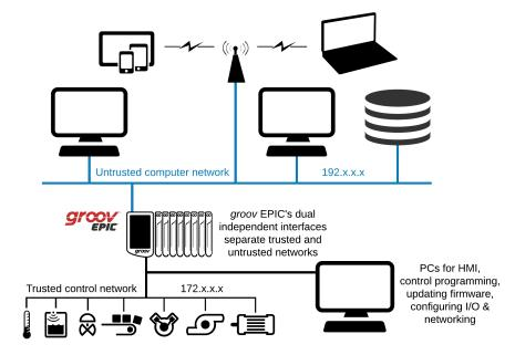
NOTE: It doesn't matter which wired interface you use for each network, except that when you first plug a groov EPIC or groov Box into the network, you must use its lower-numbered interface for initialization.
