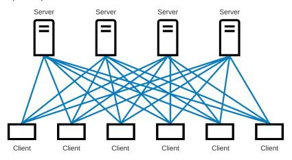
In contrast, a pub-sub architecture simplifies communications. Direct connections and repetitive requests for data are not needed. The web of links is replaced by a single link from each device to the broker. The connection between client and broker is kept open and is incredibly lightweight. Only two things travel over this connection: changed data, and a tiny heartbeat to let the broker know that the client is still there.
