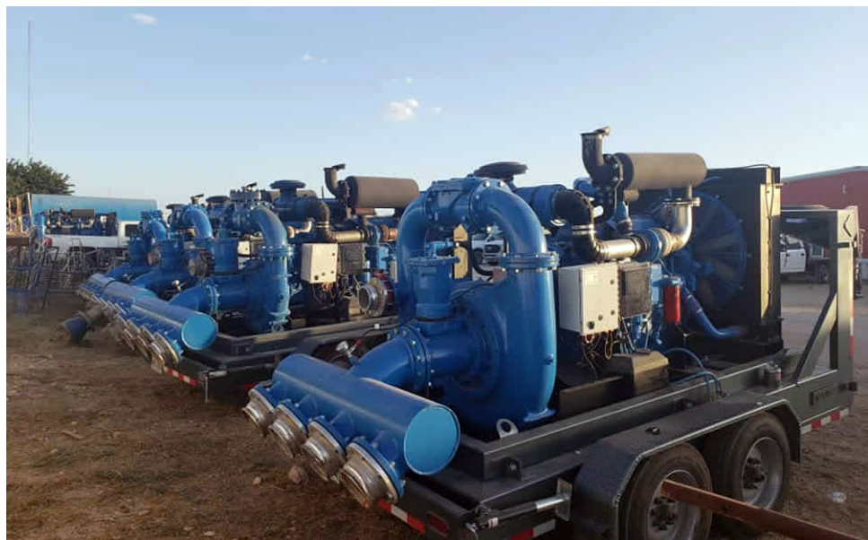
Trailer-mounted pumping units are automated with a groov EPIC processor and I/O modules.
