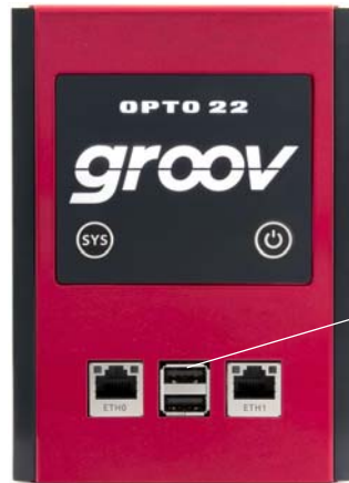
USB connectors for backing up and restoring
